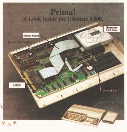
**Prima..** the high performance, low cost hard drive for Amiga 500 computers. Prima blends a large capacity, low power Quantum hard drive with the **AdIDE** host adapter for an unbeatable combination.
